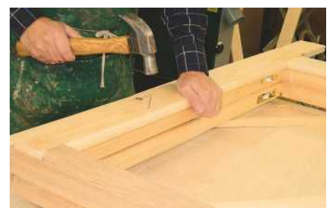
▲ Pic.22 Finally, nail the inner and outer facings together and put to one side
